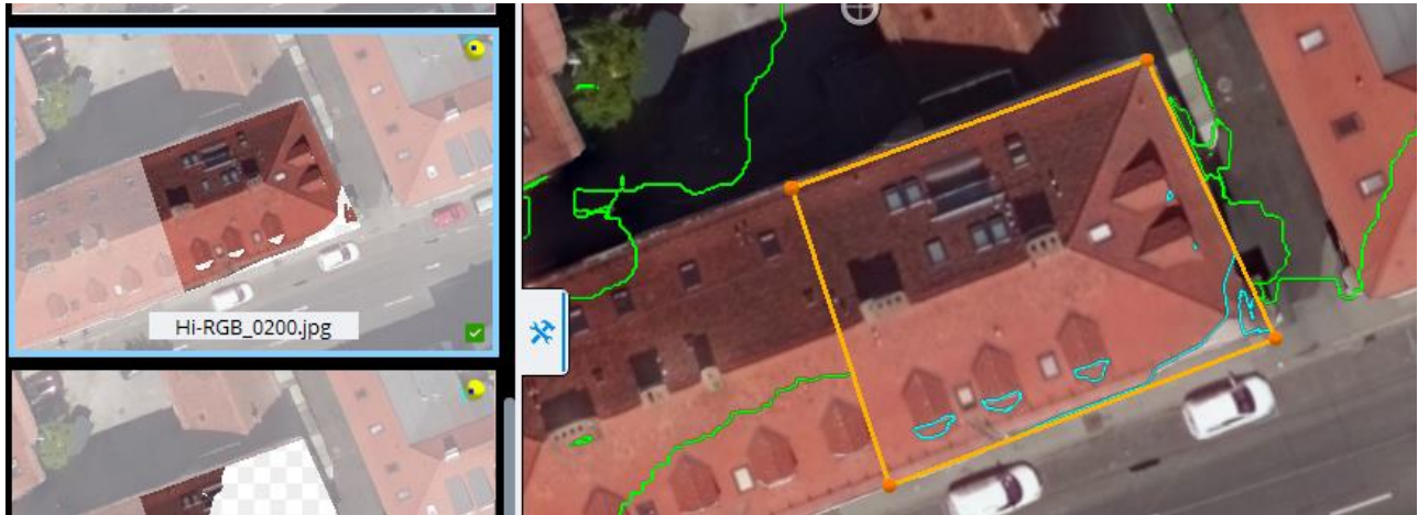
Figure 1 Green lines are the current seamlines of the orthophoto mosaic. The cyan lines are the new seamlines that will be introduced if we apply the selected image inside the polygon.
