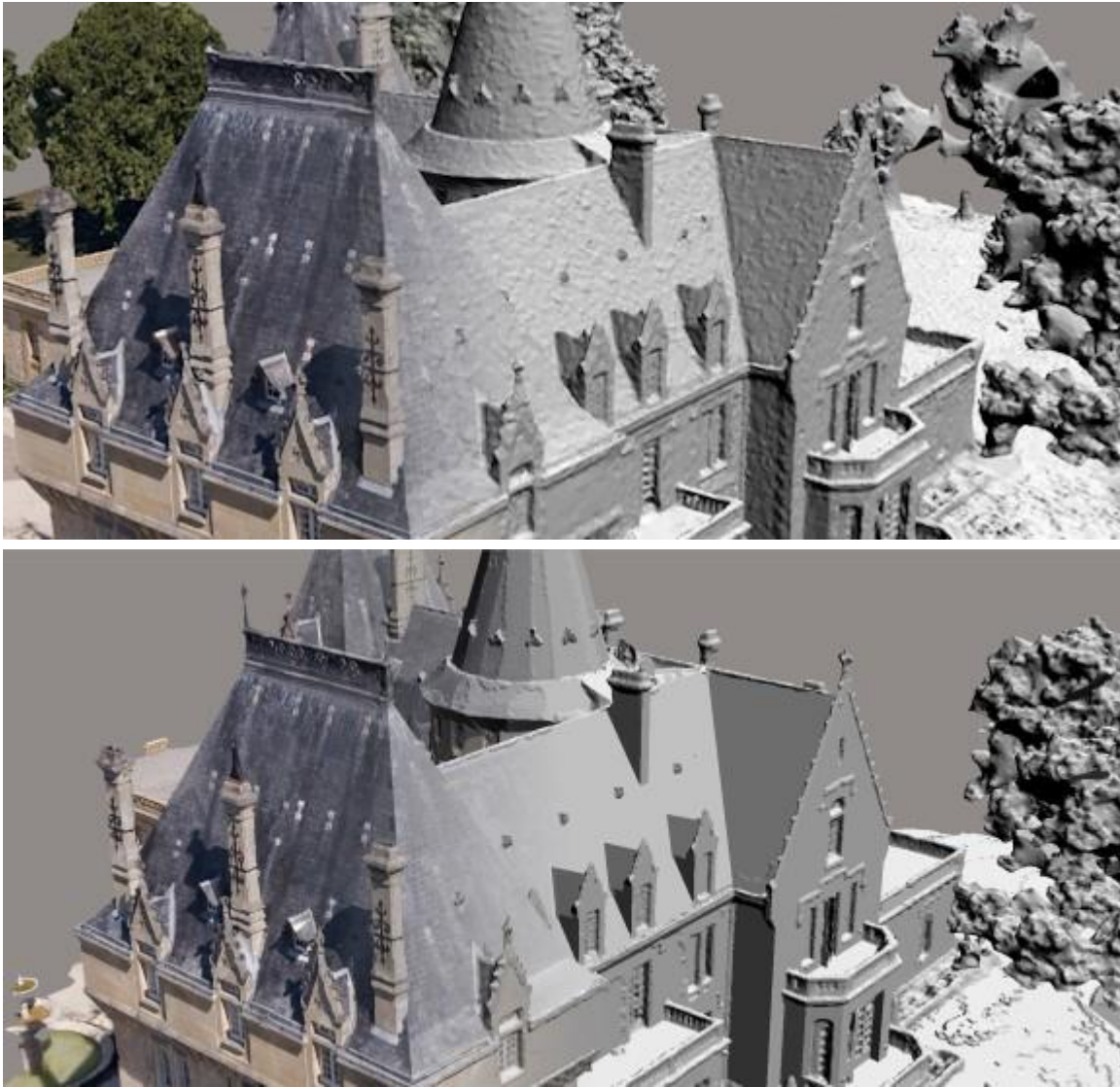
3D reconstruction of an area, without (top) and with (bottom) planar simplification.
